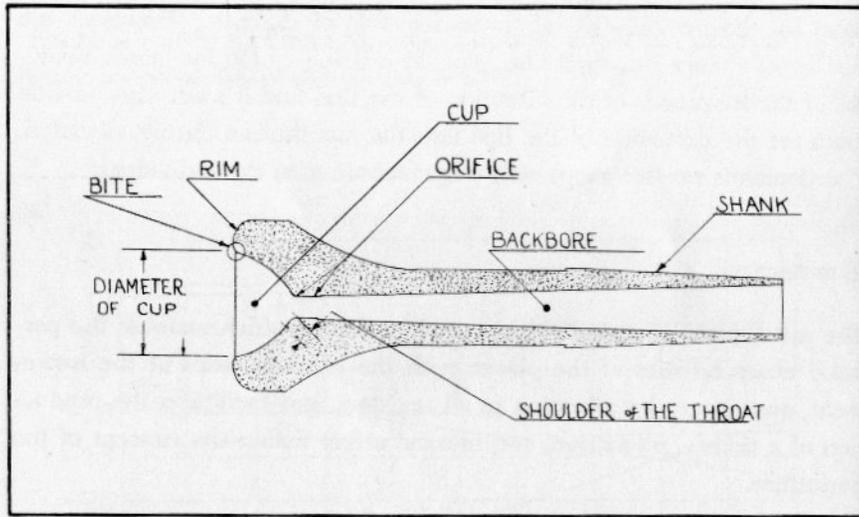
**FIGURE 4: TRUMPET MOUTHPIECE CROSS SECTION**
