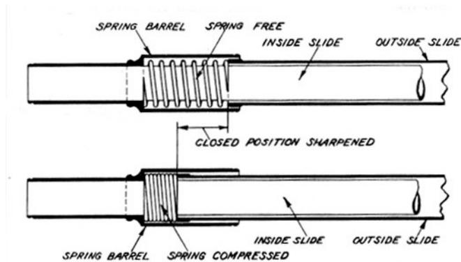
*Fig. 21—Spring barrel. Some trombones have spring barrels instead of cork barrels. This spring enables the player to favor the closed position tones. Dirt collects in the spring barrel as it does in cork barrel and fouls the action.*
