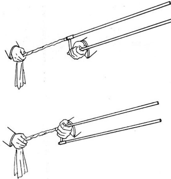
*Fig. 17—What's wrong about this picture? There are two mistakes shown. NEVER hold one slide while cleaning the other; always hold the slide you are cleaning, as in lower view. The lower view is correct except a cleaning rod is NOT recommended for the INSIDE slide. This rod may damage delicate mouthpiece. Use weighted string and cloth for inside slide. Rod is recommended for outside slide.*
