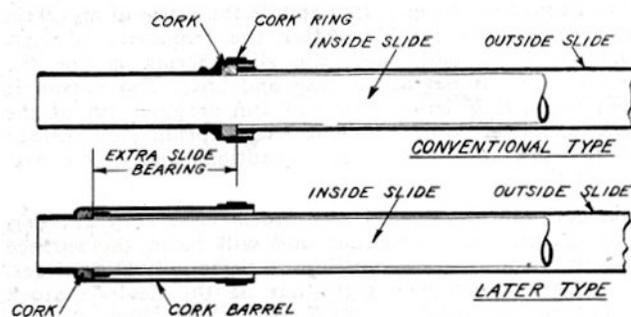
Fig. 20—Cork ring and cork barrel construction. On later models providing for longer outside slides which run up into cork barrel, dirt collects in cork barrel. This dirt is loosened when slides are oiled and the dirt is dragged out onto the slides where it fouls the action. For outside slide length, see also Fig. 14.
