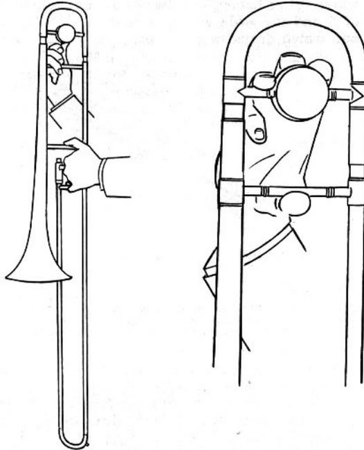
*Fig. 22—Changing tuning slide. Force applied in center of braces will avoid advancing one side of slide beyond the other and causing the slides to cock and stick. Left, opening; right, closing.*
