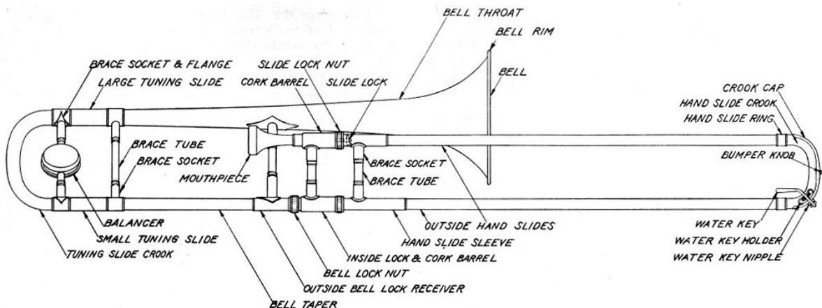
Fig. 11 — Tenor Slide Trombone, with tuning in bell. Equipped with slide lock and bell lock.
