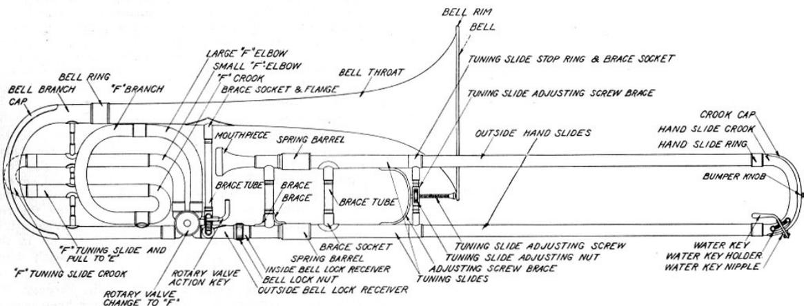
Fig. 12—Bass Slide Trombone, with rotary valve to F and slide to E. Tuning is in slides.
