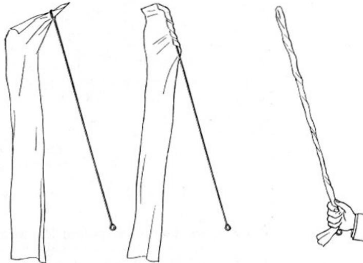
**Fig. 16—How to cover trombone cleaning rod. Use piece of cheesecloth 6 to 8 inches wide and 5 to 6 feet long. Don't simply thread the cloth through eye of rod. First insert corner in eye, then twist rod until cloth covers entire length. Hold end of cloth tightly in hand to keep cloth from sliding and bunching when you run the rod through the slide.**
