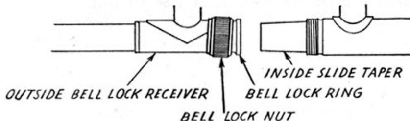
*Fig. 15—Slide-to-bell lock. In taking slides from bell, be sure bell lock nut is completely unscrewed, or bell lock ring may be torn off or damaged when friction fit of inside slide taper is broken loose.*
