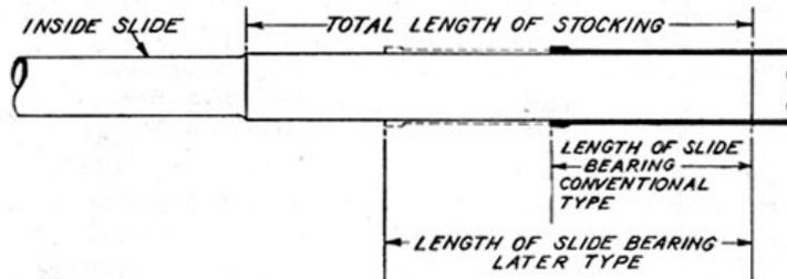
*Fig. 14—Trombone inside slide and stocking, with outside slide in solid black. The outside diameter of the stocking is only .006" less than the inside diameter of the outside slide. This makes a clearance on a side between the stocking and outside slide of only .003" or the diameter of a human hair. Dotted lines show outside slide is longer on present models than on old type trombones. See also Fig. 20.*
