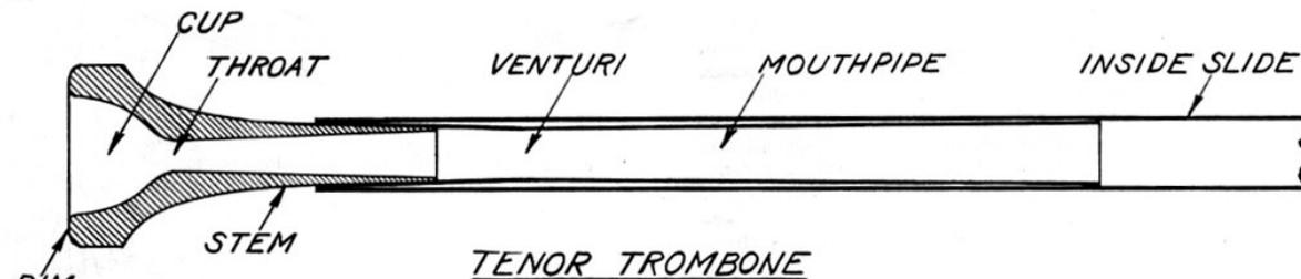
Fig. 19—Trombone mouthpiece and mouthpipe. Note mouthpipe inserted inside the inside slide. Do NOT use cleaning rod for inside slides, for you are liable to damage this thin mouthpipe. The venturi of the mouthpipe is one of the most critical spots in the trombone and if it becomes enlarged through the use of a rod, the response of the trombone will be impaired.
