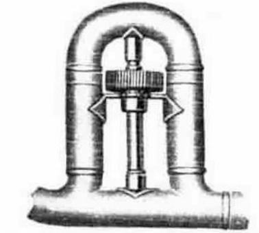
**A**BOVE we illustrate the tuning mechanism which is found on all “Victor” Cornets. This is a patented feature and while it is extremely helpful to the player it is also very simple and there is nothing to get out of order. Tuning is accomplished by turning the knurled wheel. Causing the slide to come out lowers the pitch, and causing the slide to go in raises the pitch.
